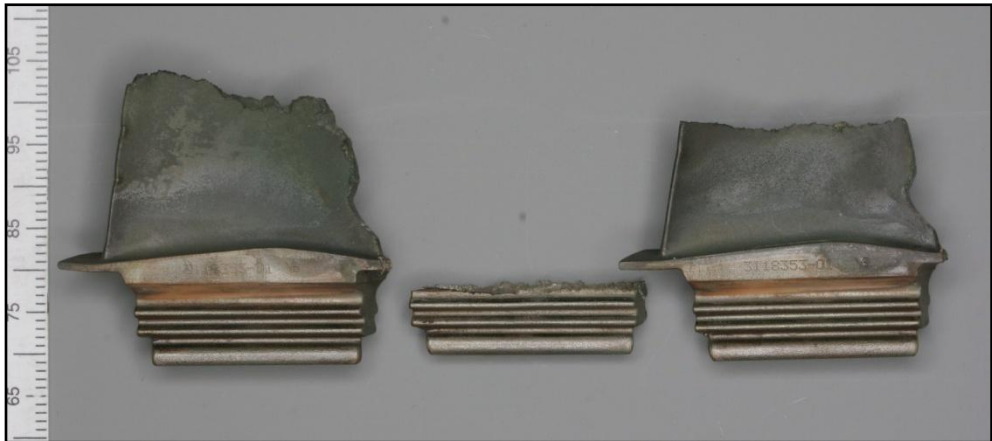
Figure A11: Blades removed from the second-stage power turbine disk
