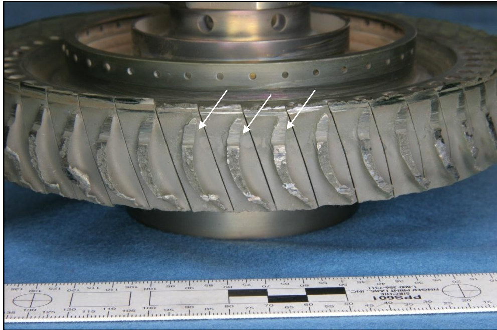
Figure A9: Rotational wear damage to the blade leading edge transition (arrowed) – result of interference with the stator ring
