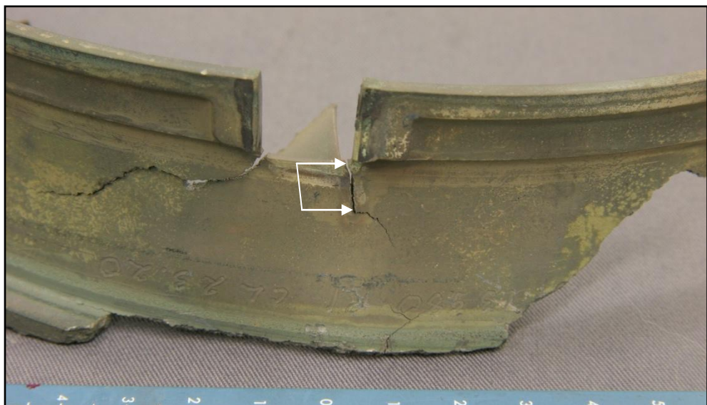
Figure A4: Suspected prior cracking of stator ring – between arrows
