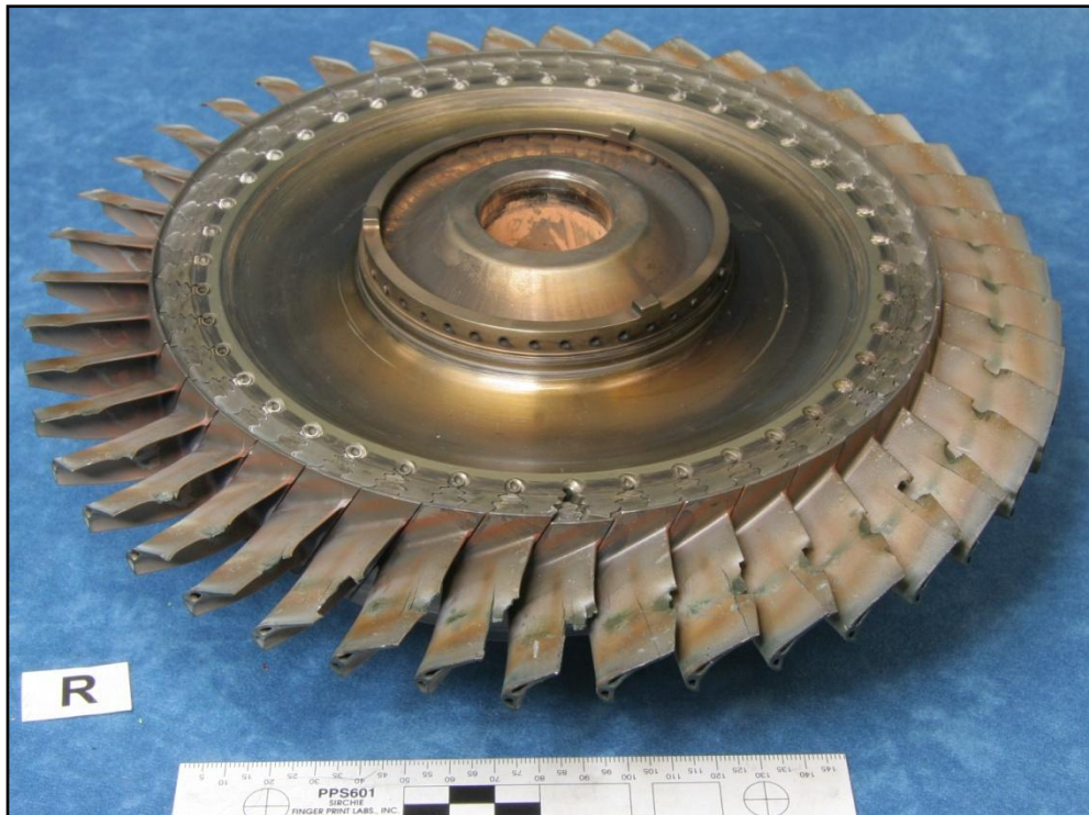
Figure A7: Suspected hard-object impact damage to compressor turbine blade trailing edges (arrowed)
