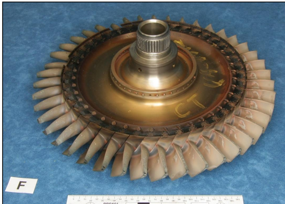
Figure A5:Upstream face of the engine compressor turbine disk
