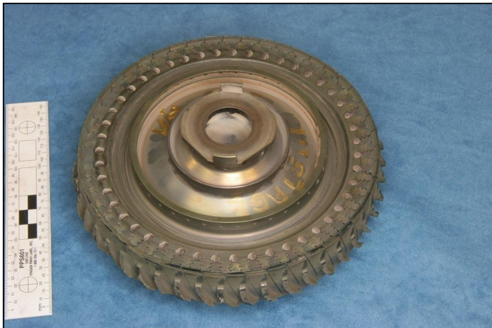
Figure A8: First stage power turbine disk and fracture blade set
