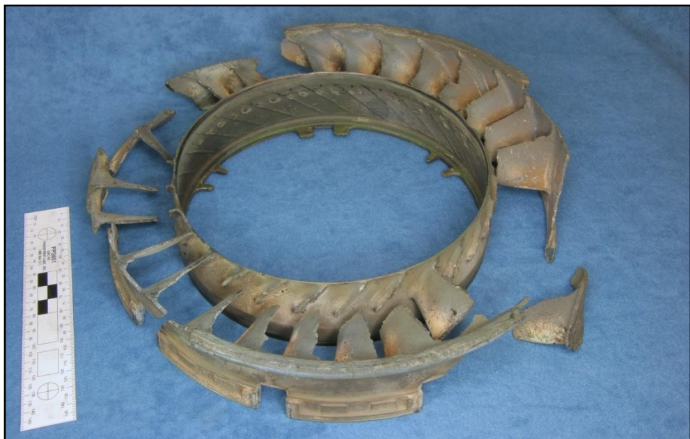
Figure A4: Suspected prior cracking of stator ring – between arrows
