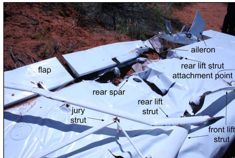
Figure 8: Wing and aileron damage
