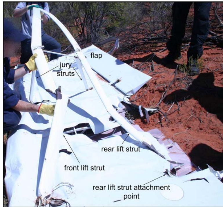
Figure 8: Wing and aileron damage
