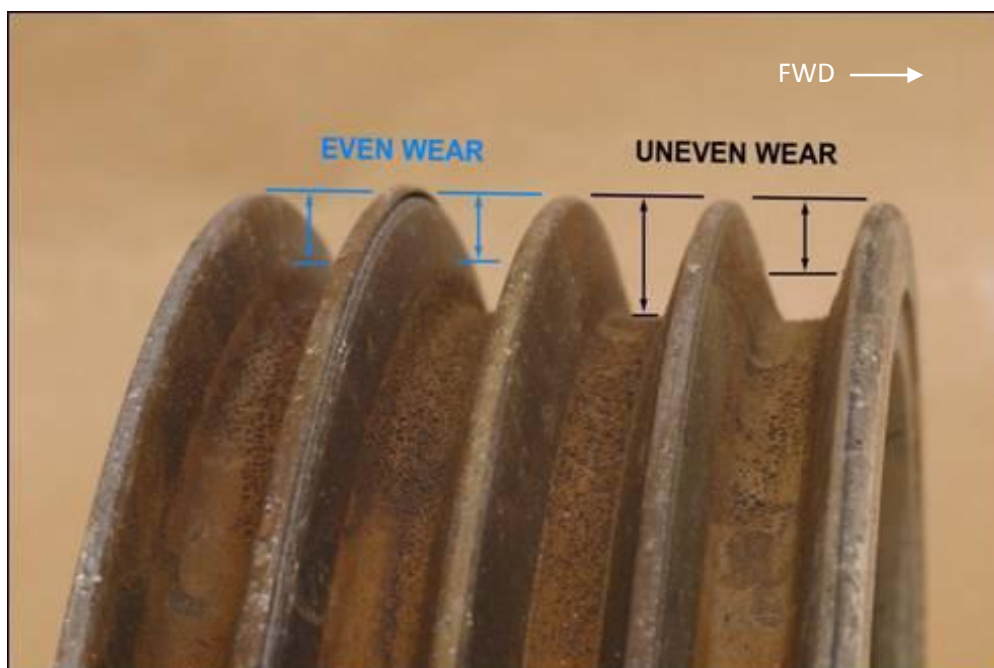
Figure 8: Upper sheave wear pattern
