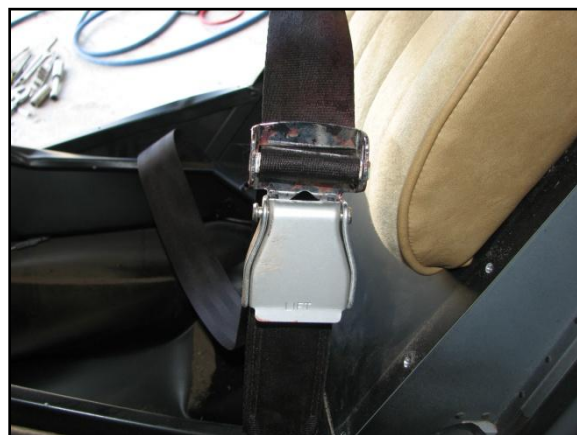
Figure 7: Combined seat belt and inertia-reel shoulder strap.
