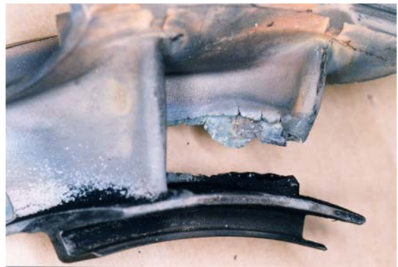
Fig. 17. Destruction of a guide vane from the effects of overheating and oxidation.
