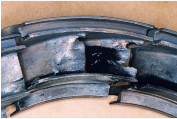
Fig. 14. Mechanical damage to the trailing edges of the inlet guide vanes (typical).
