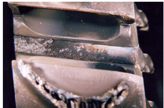
Fig. 3 (Top left). Failure of the turbine blade from beneath the platform base.
