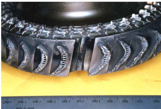
Fig. 1. Forward face of the stage-one turbine wheel – missing blade indicated.
