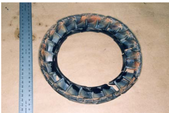
Fig. 12. Turbine inlet guide vane segments – forward faces.
