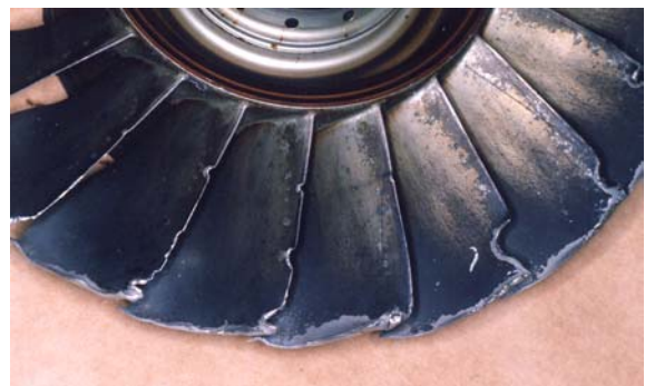
Figure 6. Dark deposit on the forward faces of the blisk aerofoils.
