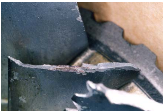
Figure 9. General view of the fractured blade lower section.
