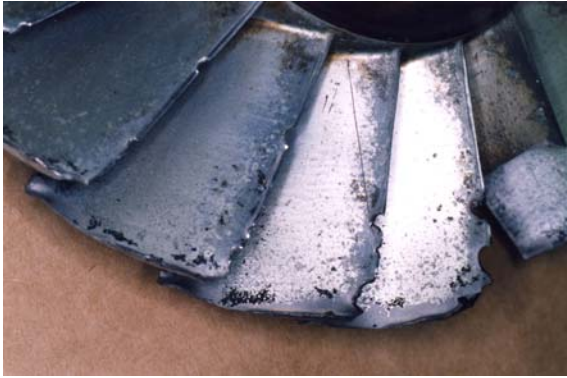
Figure 7. Forward (convex) aerofoil faces after cleaning. Bright finish is typical of a metallic coating.
