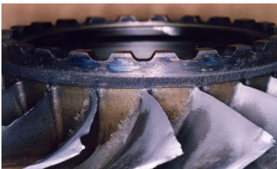
Figure 5. Evidence of mechanical 'rub' on the rear edge of the blisk hub.
