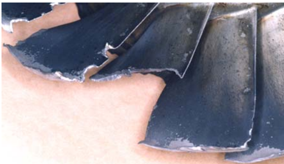
Figure 3. Fractured blade and mechanical damage to other blades.
