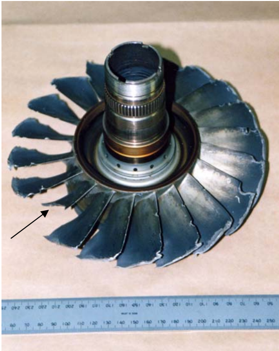
Figure 1. Blisk front view – fractured blade is arrowed.
