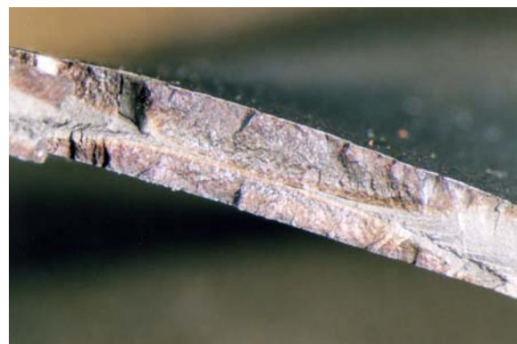
Figure 10. Closer view of the semi-elliptical stained regions at the mid-chord position.
