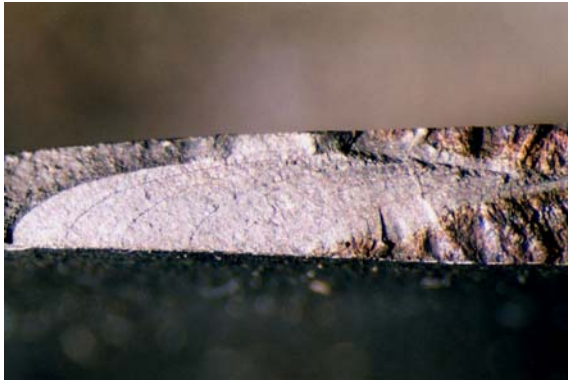
Figure 11. Clear crack arrest marks extending out from the central stained region.
