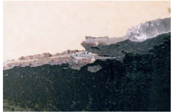
Figure 12. Progression of fracture on two adjacent planes, forming a step feature.
