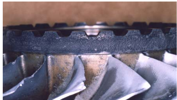
Figure 4. Erosion damage to rear edge of blisk hub.
