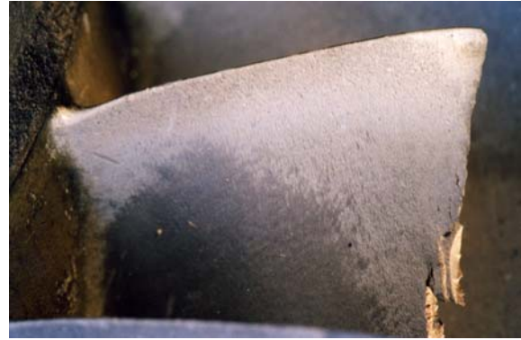
Figure 8. Rear (concave) face of an aerofoil showing the typical eroded appearance.
