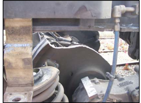
Figure 2: SCT 008 fractured locomotive wheel L4.
