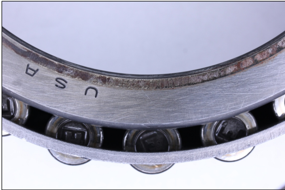
Figure 8: Fretting wear (inboard cone)
