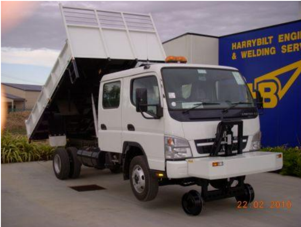
Figure 6: Hirail 3 with rail guidance wheels lowered
