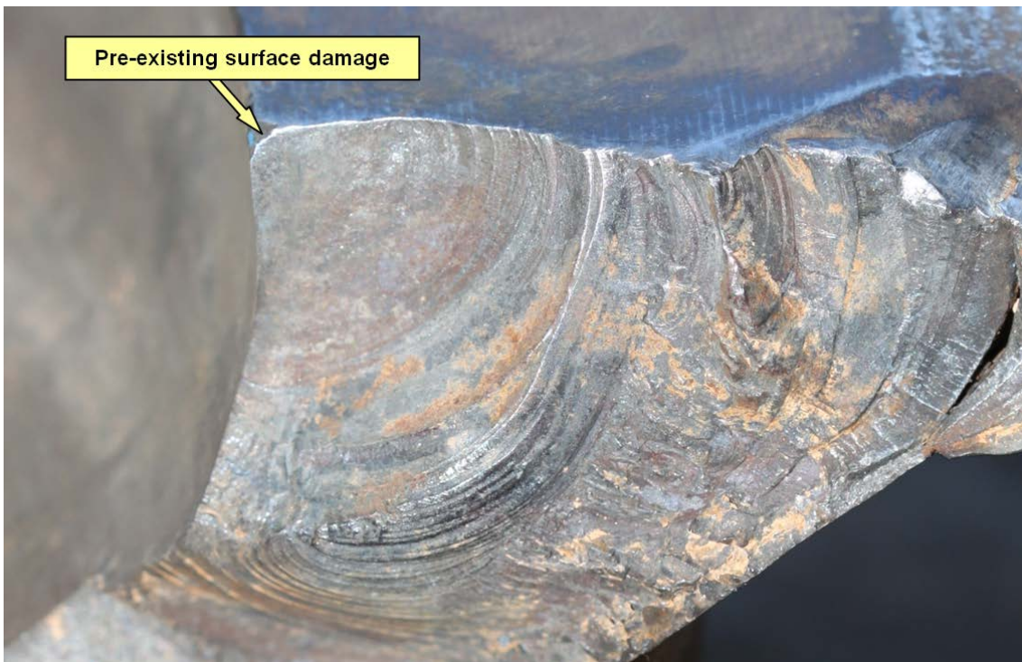
Figure 10: Detached section (A) showing pre-existing surface damage on corner of back rim face and radial propagation point of the fatigue crack
