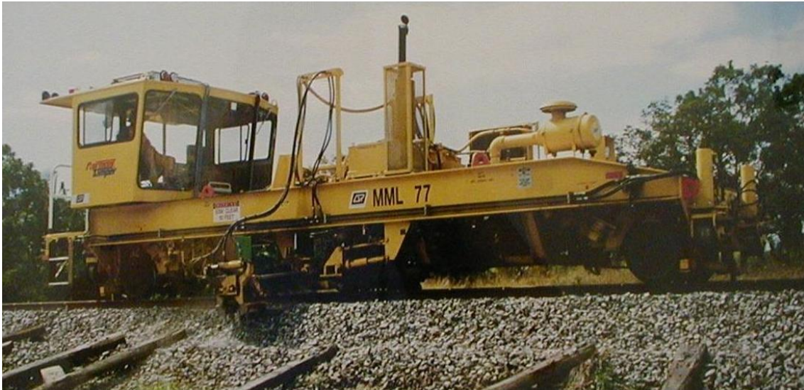
Figure 23: Fairmont Tamper RT10 Tie Exchanger
