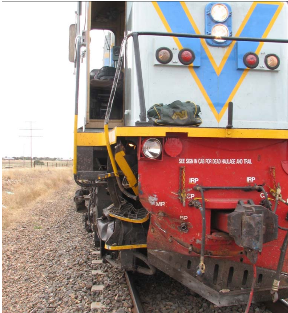
Figure 7: Photo of locomotive, NA1874, showing extent of damage.
