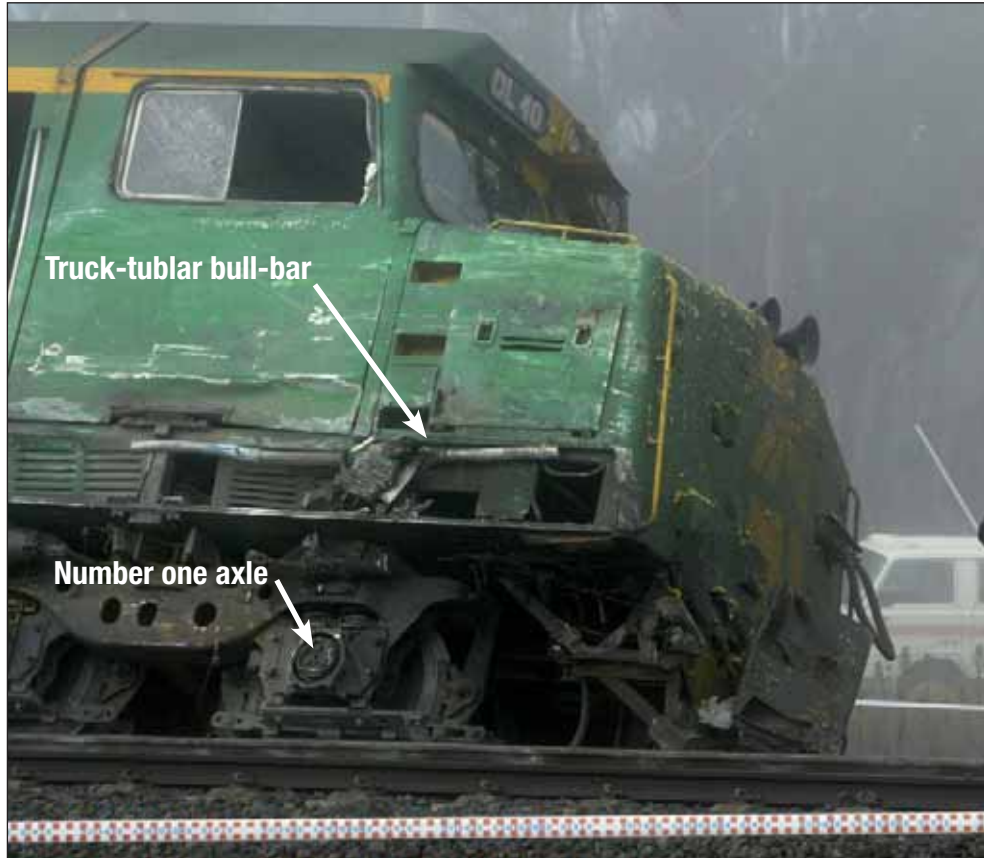
Figure 7: Tubular bull-bar imbedded in DL 40
