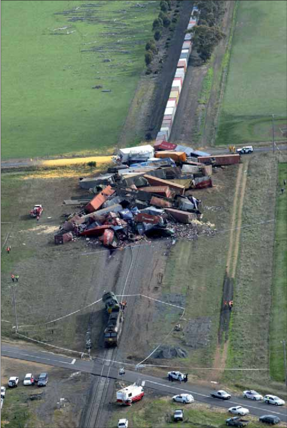
Figure 8: Compressed wreckage of train 4AM3
