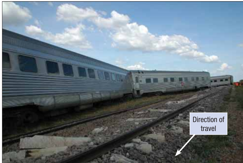
Figure 22: The Ghan carriages jack-knifed, northern side of the track
