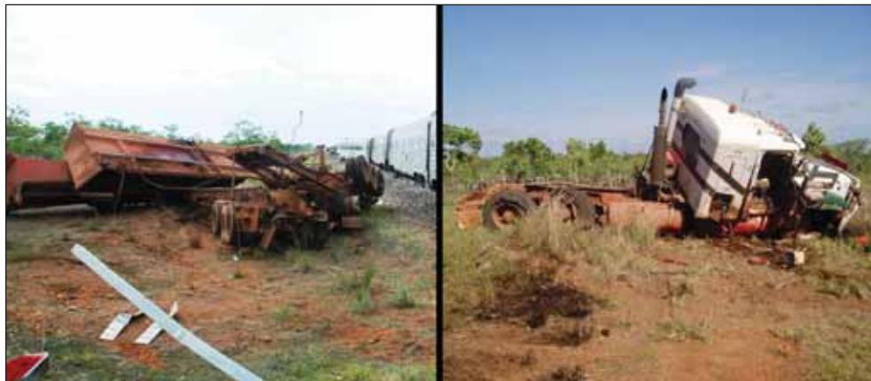
Figure 13: Damaged prime-mover (right) and trailers (left)
