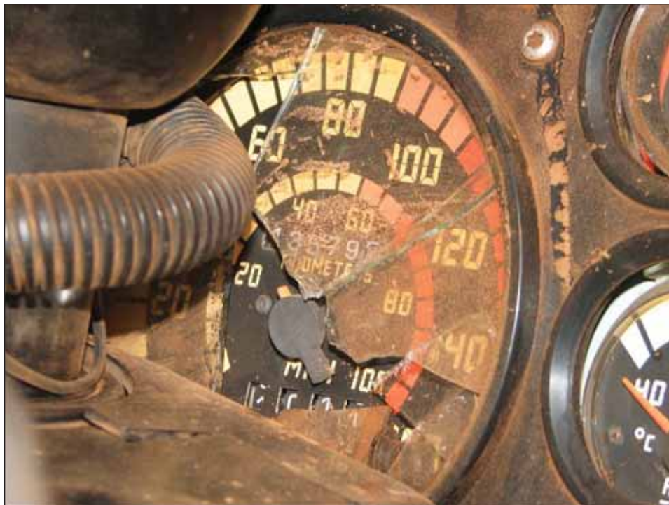
Figure 17: Truck speedometer jammed at about 50 km/h
