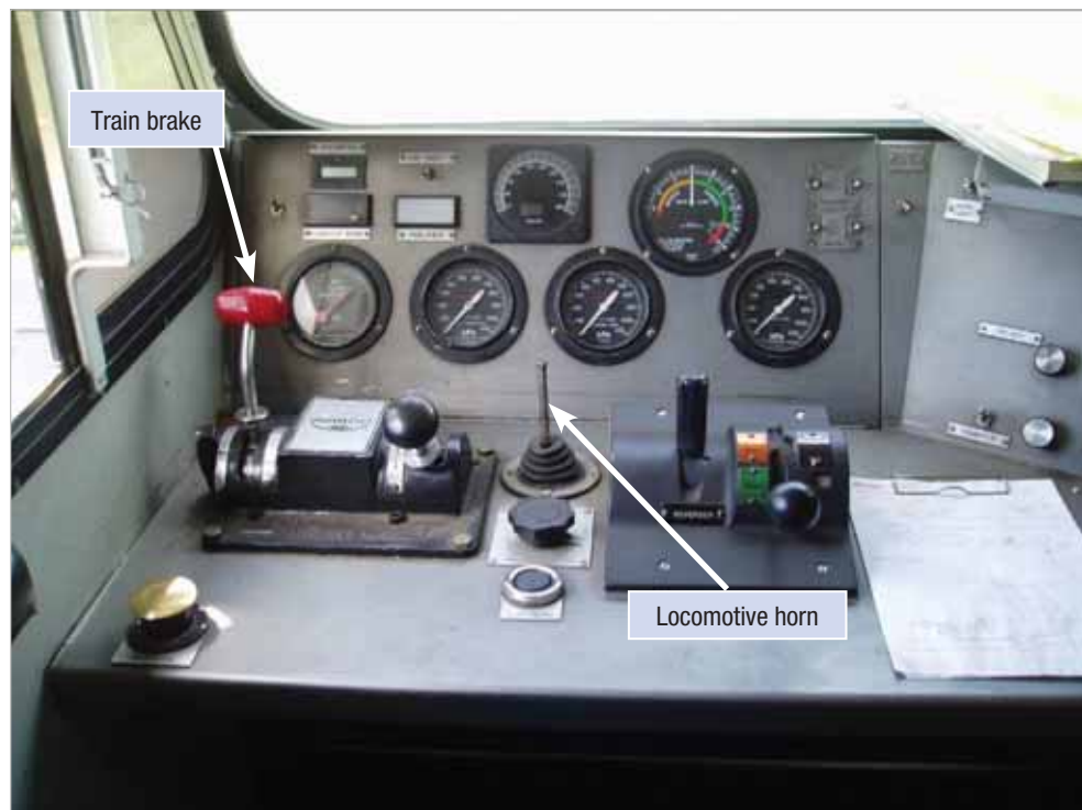
Figure 4: Driver controls, AN 5
