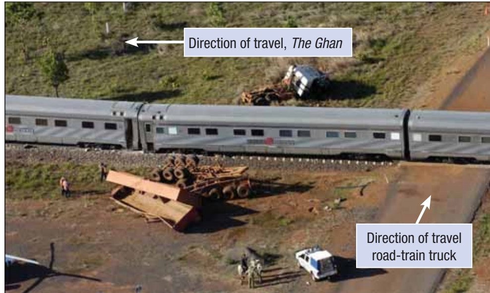
Figure 8: Separation of prime-mover and trailers
