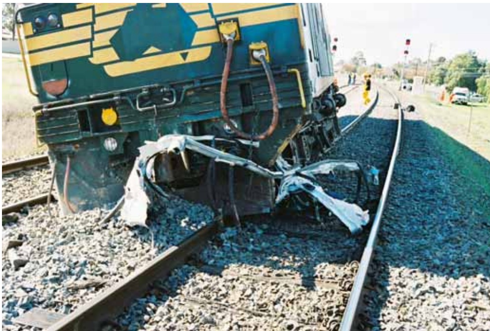
Figure 5: Damage to the points-machine, caused the locomotive to derail. Part of the motor vehicle remained wedged in the locomotive coupler. (Photograph, courtesy of Victoria Police).
