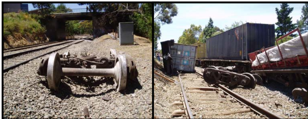
Figure 15: The first bogie to derail (left), approximately 2km prior to the final location of derailed wagons (right)
