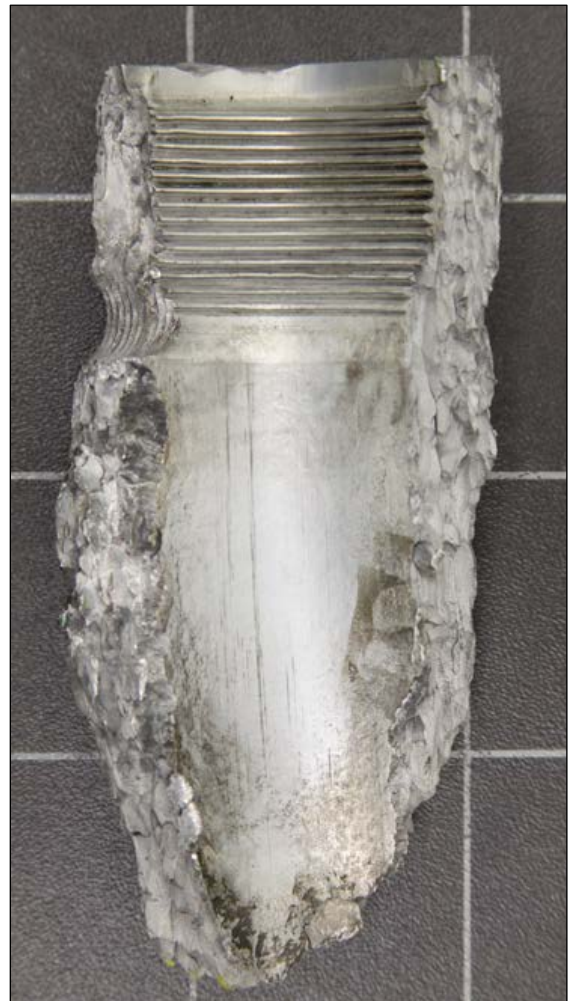
Figure 6: Section of fractured discharge tube
