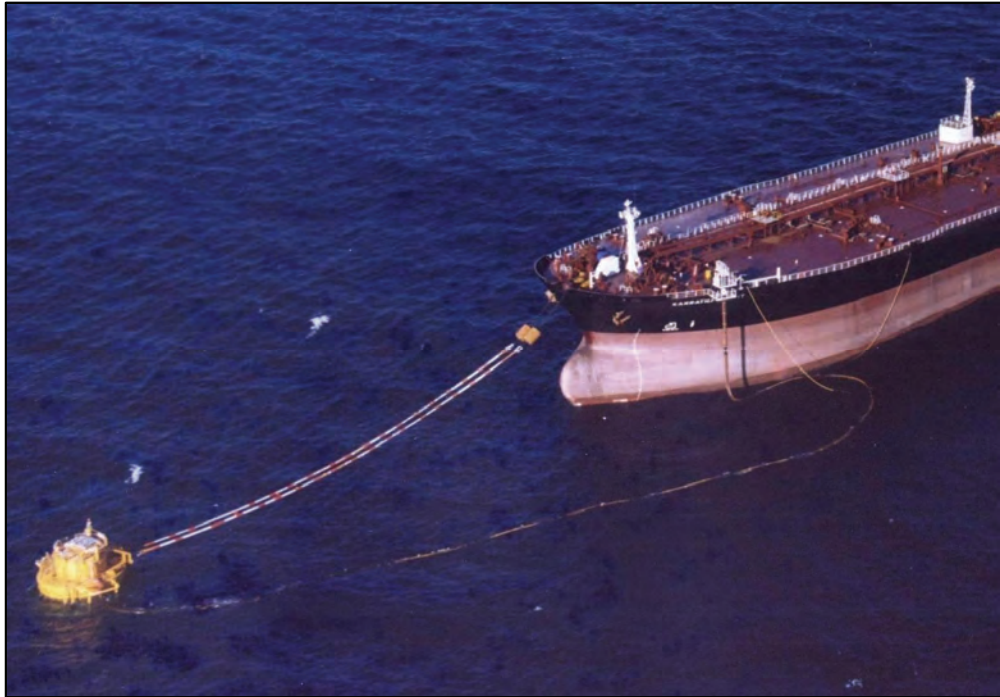
Figure 3: Karratha Spirit's hawsers and import hose at the CALM buoy
