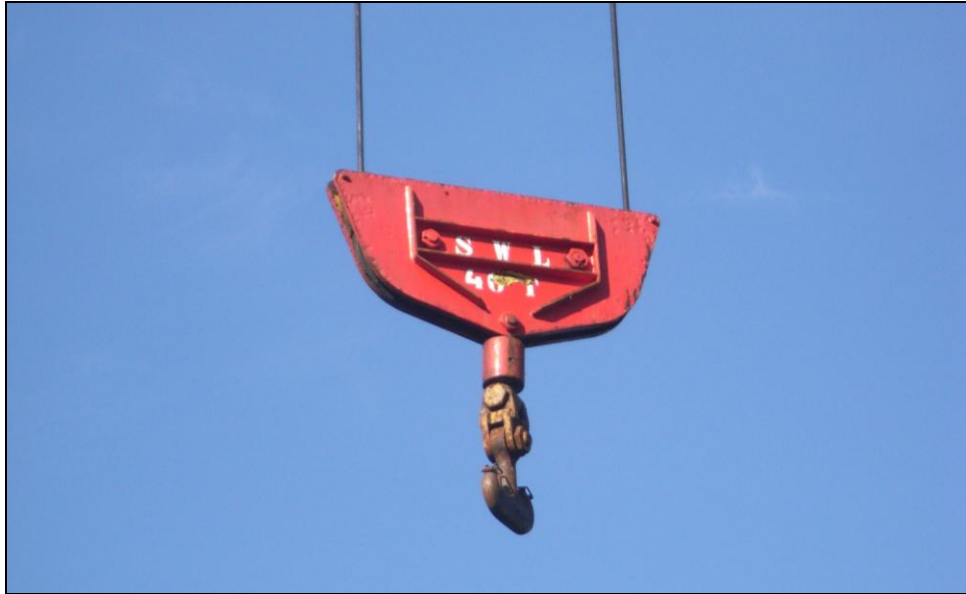
Figure 2: The block and rams-horn hook assembly
