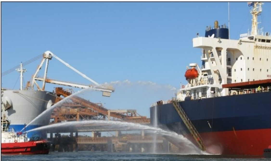
Figure 4: Harbour tug boundary cooling the engine room
