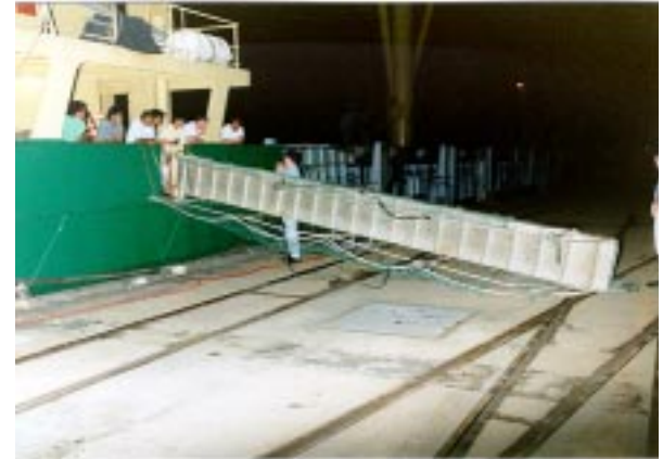
Tipped gangway shortly after the incident
