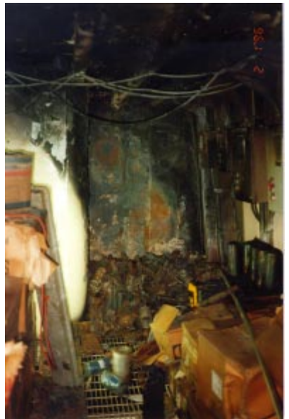
Starboard forward upper corner of reel room after the fire had spread to stored filters in cardboard boxes.
