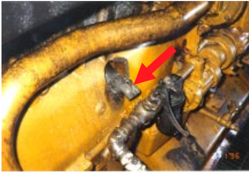
Side of Caterpillar D343 crankcase showing bottom of N0.4 connecting rod.
