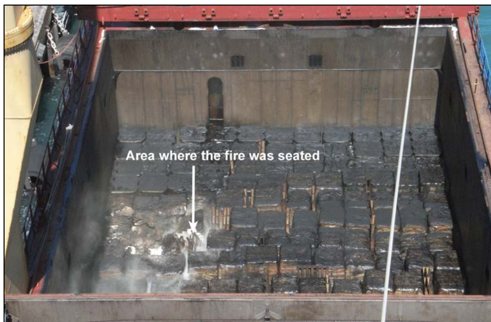
Figure 3: The aft cargo hold after the smoke had cleared.
