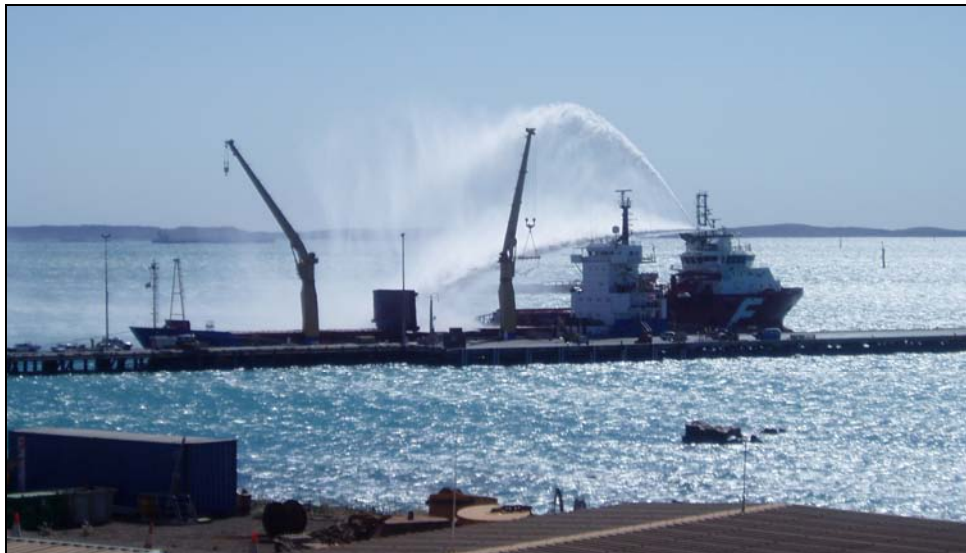
Figure 5: Far Sword's fire monitor being used to extinguish the fire
