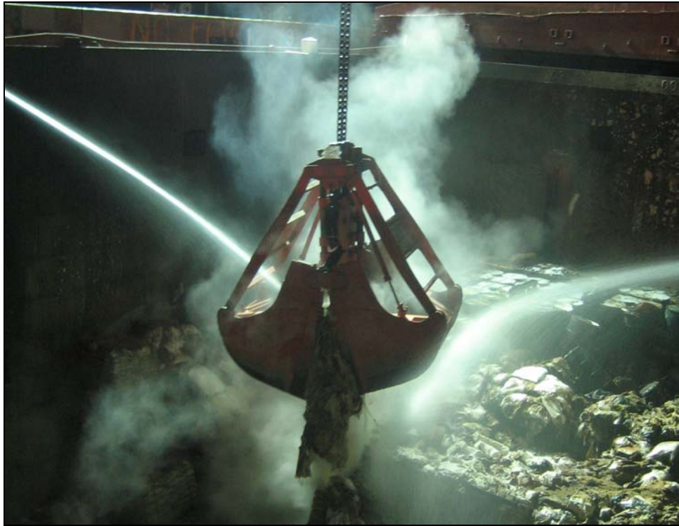
Figure 7: Removing the hot spots of cargo
