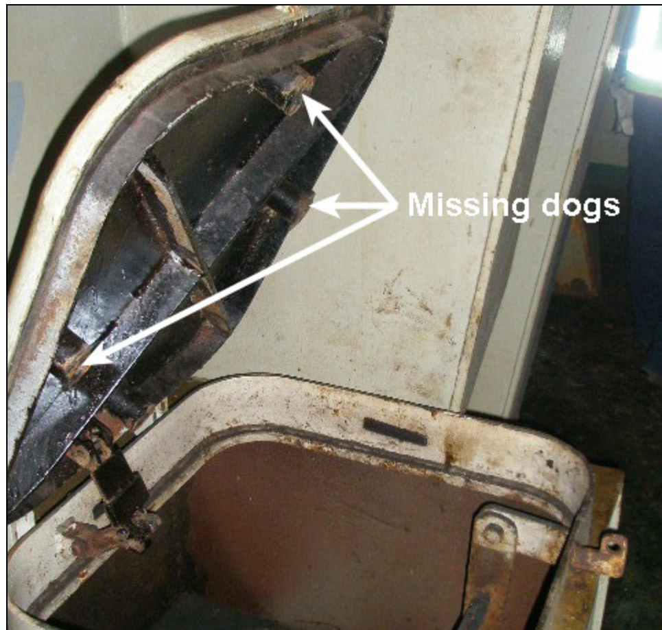
Figure 12: Hatch with missing dogs
