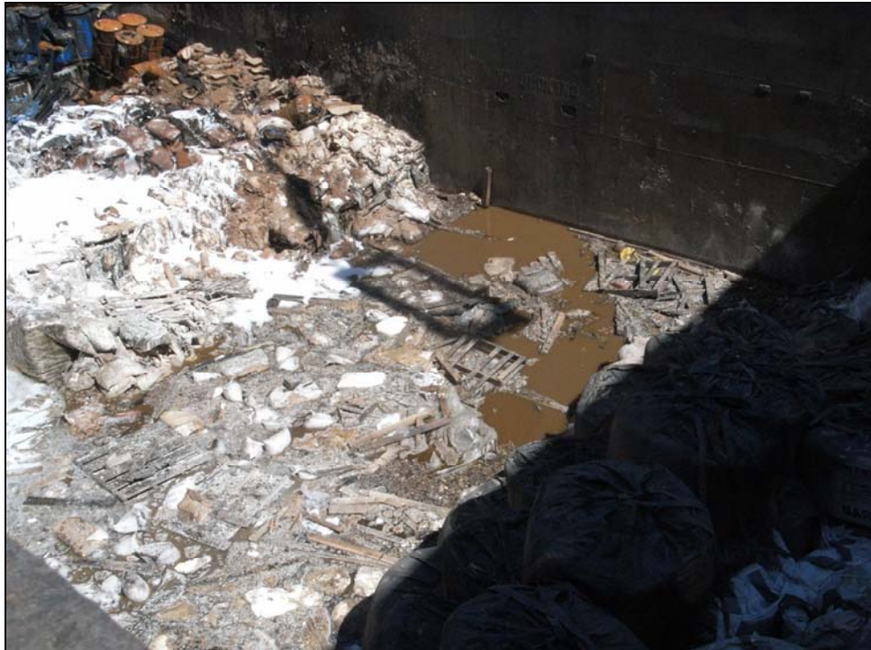
Figure 6: The hold flooded with liquid to a depth of about two metres.
