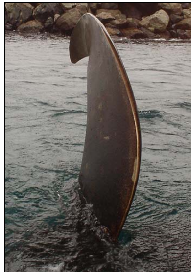
Figure 8: Most bent blade
