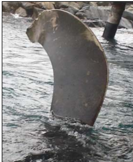
Figure 7: Most damaged blade
