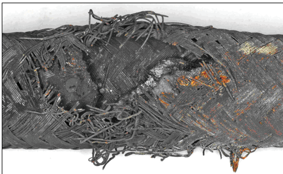
Figure 10: Close-up of the filter hose's wire braid wear
