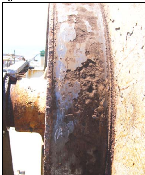
Figure 11: Corroded winch brake drum
