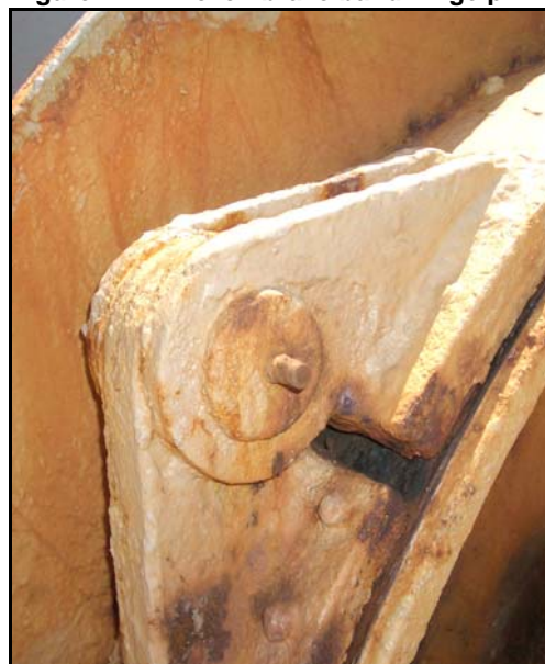
Figure 12: Frozen brake band hinge pin
