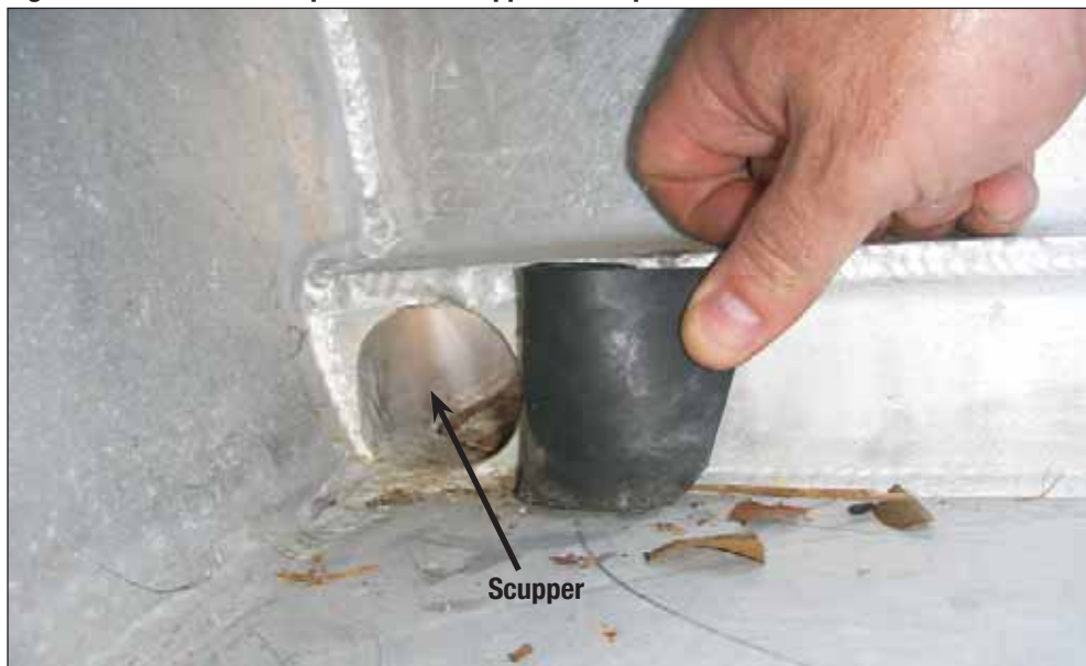
Figure 16: Port side cockpit transom scupper and flap
