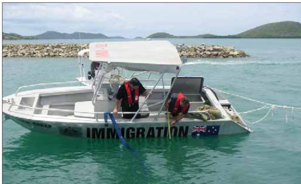
Figure 11: Measurement of lowest freeboard during static stability test
