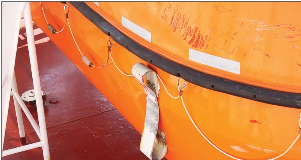
Figure 8: Port lifeboat's contact damage
