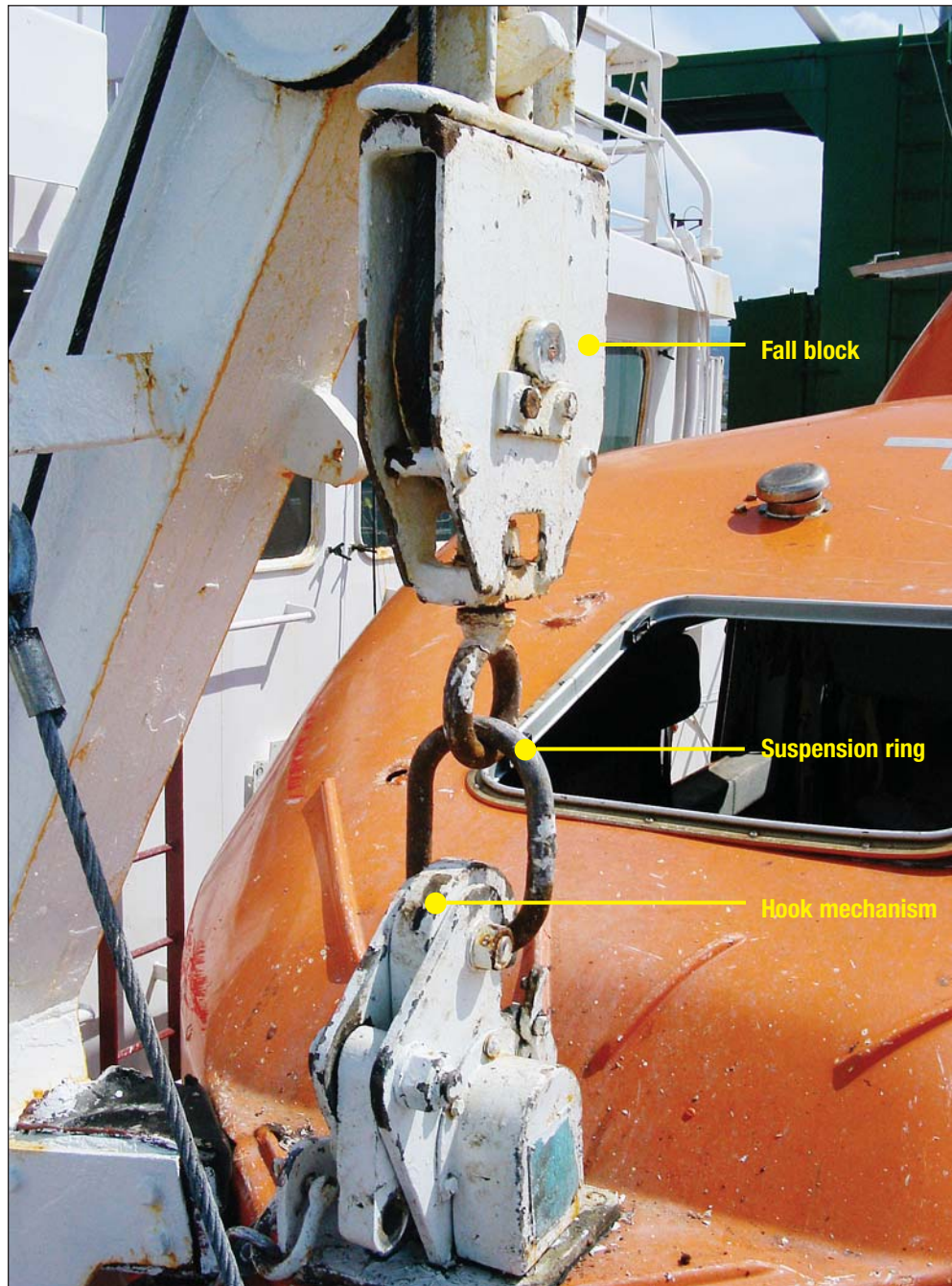
Figure 14: Port lifeboat's forward lifting assembly
