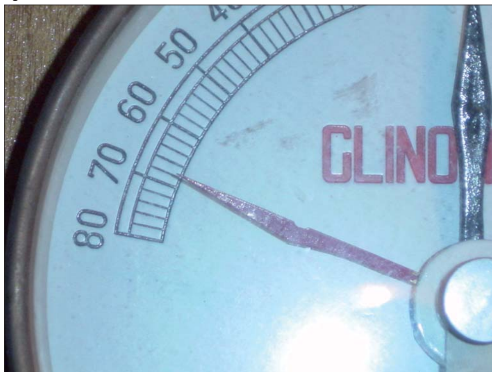
Figure 4: Inclinometer mounted on the aft bulkhead of the master's cabin
