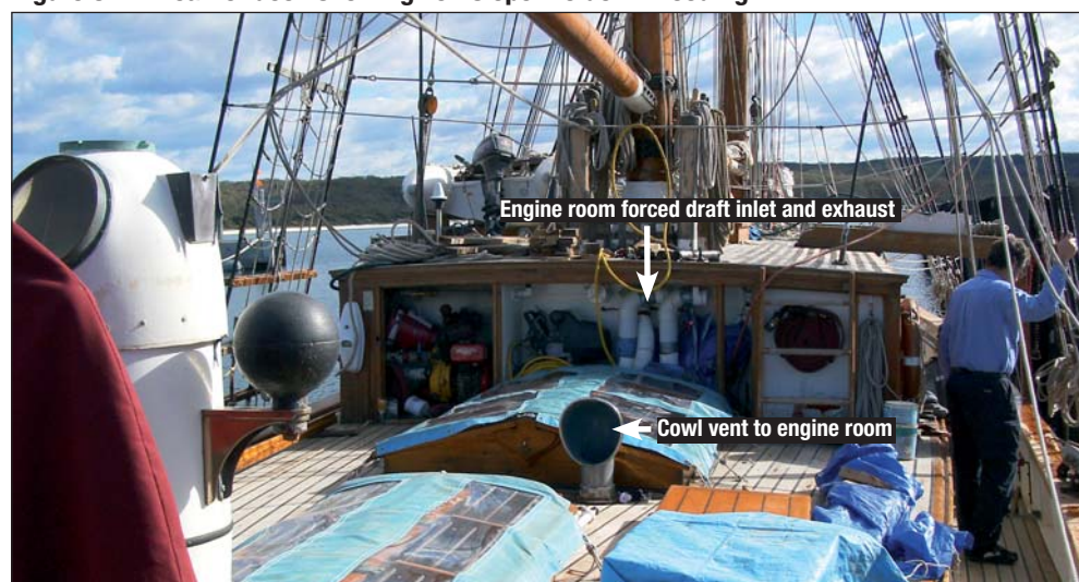
Figure 8: Weather deck showing vents open to down flooding
