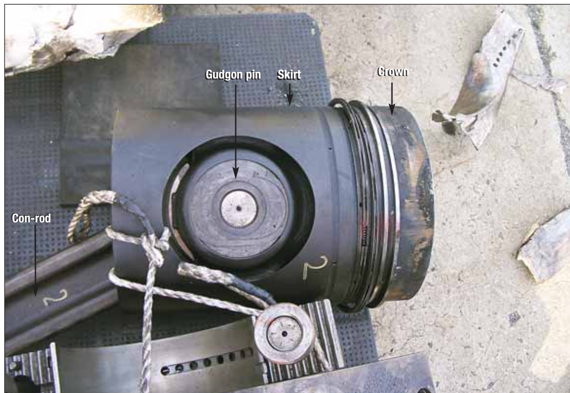
FIGURE 2: Piston assembly on pallet
