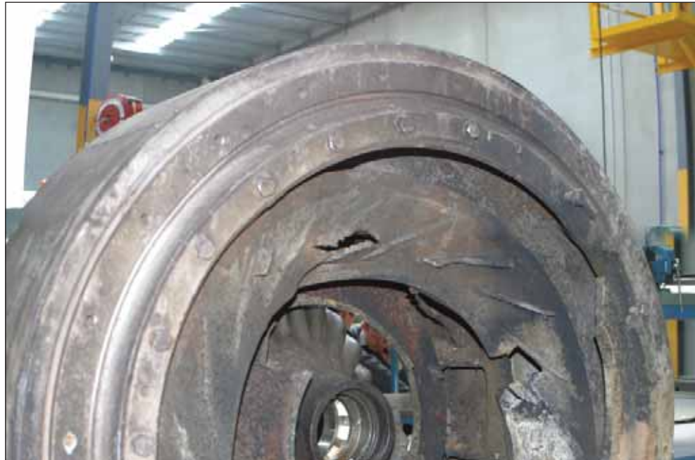
Figure 11: Looking into the remnants of the compressor housing
