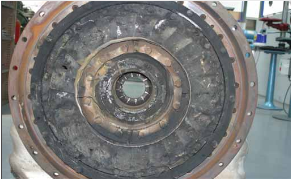
Figure 3: Heavy impact damage to the otherwise intact turbine nozzle ring
