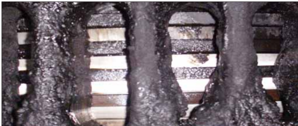
Figure 8: Number one cylinder liner scavenge ports (scavenge manifold side)
