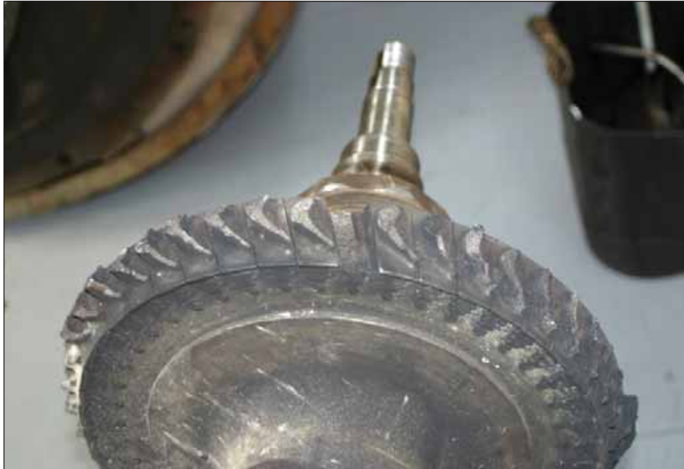
Figure 6: 'Cobbed' turbine rotor with all blades fractured
