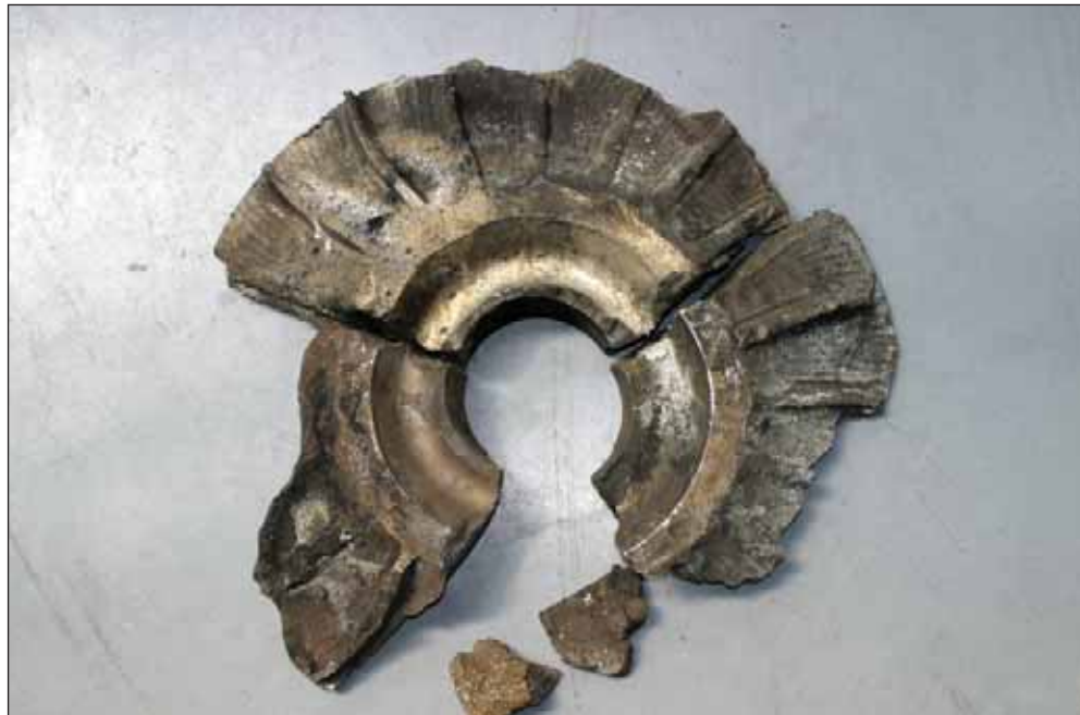
Figure 9: Recovered segments and fragments of the impeller disc
