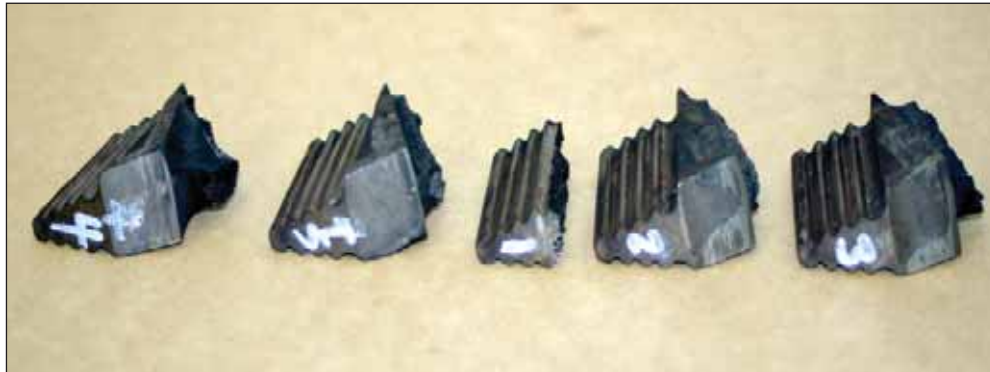
Figure 13: Selection of turbine blades taken from around the blade that failed at the fir-tree root
