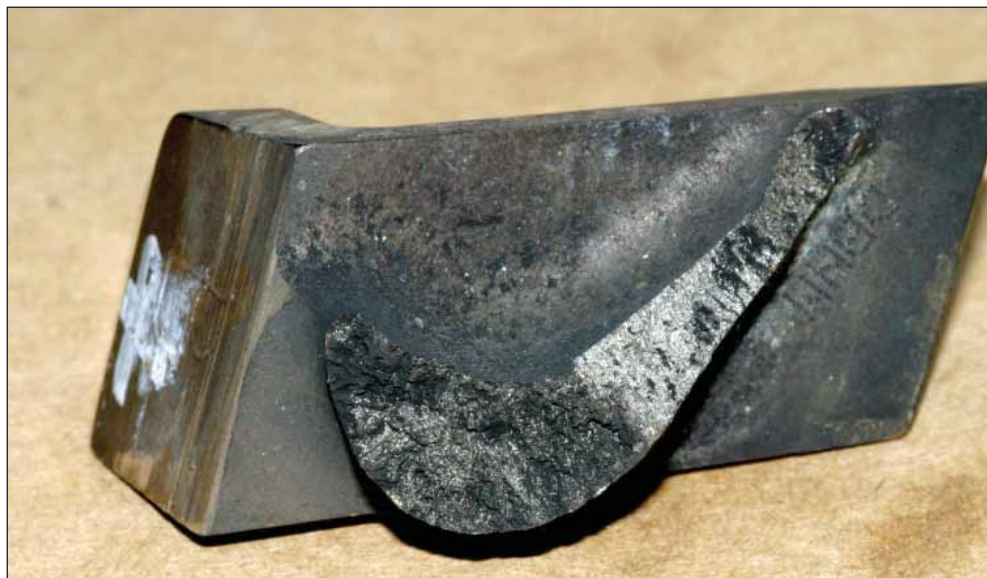
Figure 14: Carbonaceous, sooty deposit over a turbine blade fracture surface
