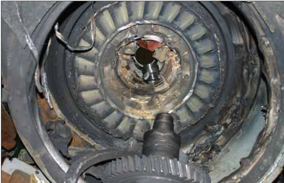
Figure 27: Intact nozzle ring and guide vanes
