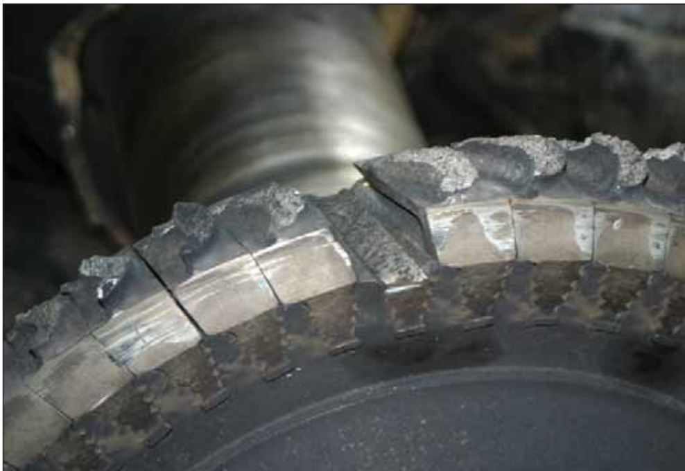
Figure 7: Left shingle turbine blade fractured at the top of the fir-tree root
