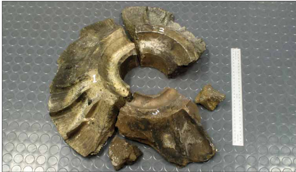
Figure 17: Segments and smaller fragments of the compressor impeller disc. Note the predominant radial orientation of the primary fractures
