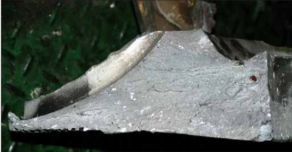
Figure 32: Typical brittle overload fracture exhibited by the impeller disk
