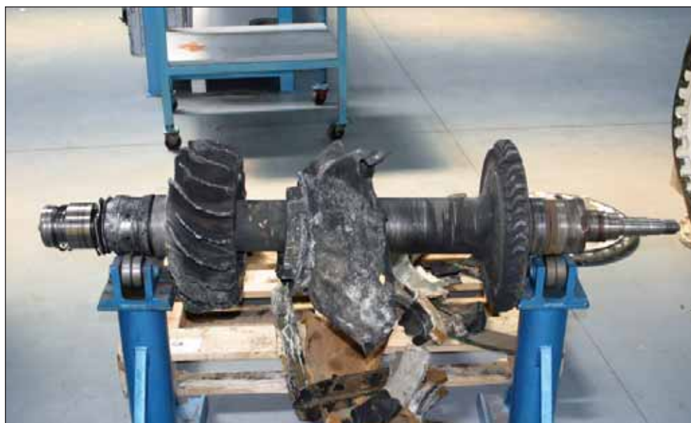
Figure 5: Turbocharger shaft with (left to right) inducer, missing impeller disc, partition and turbine disc
