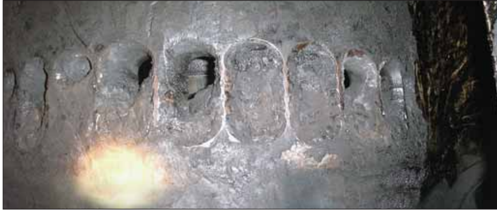
Figure 10: Number three cylinder liner scavenge ports (scavenge manifold side)
