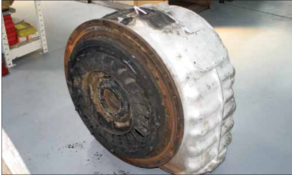
Figure 2: Exhaust inlet casing and turbine nozzle ring
