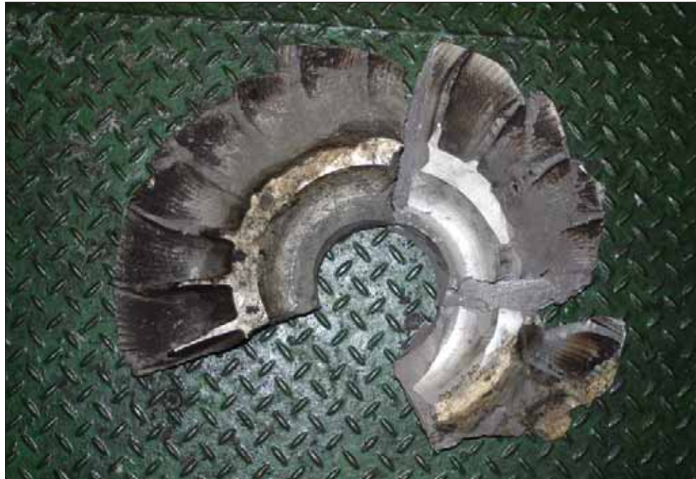
Figures 30 & 31: Segmented failure of the compressor disk, very similar to the first failure (fig.17)
