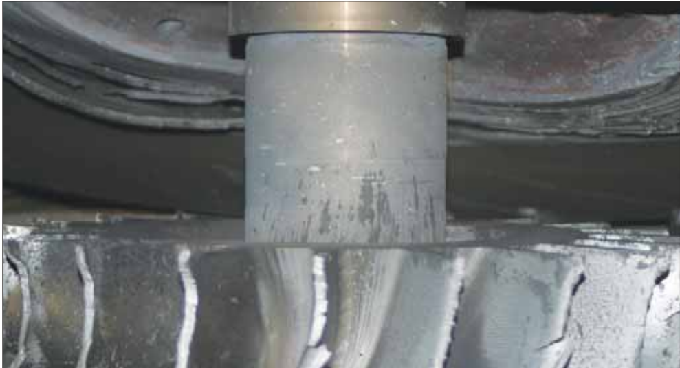
Figure 33: Shaft surface showing no evidence of impeller insecurity or rotation
