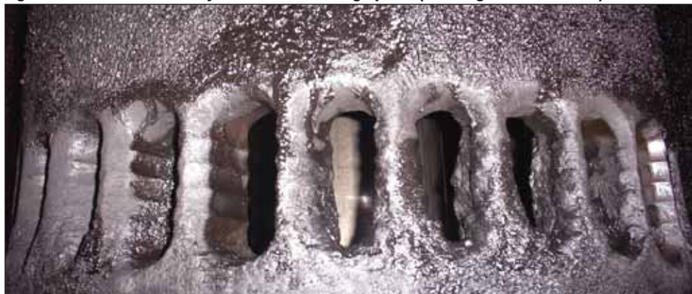
Figure 12: Number five cylinder liner scavenge ports (scavenge manifold side)
