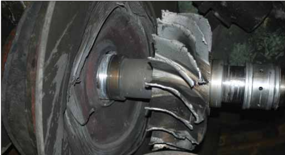
Figure 34: Inducer in place adjacent to the normal disk location
