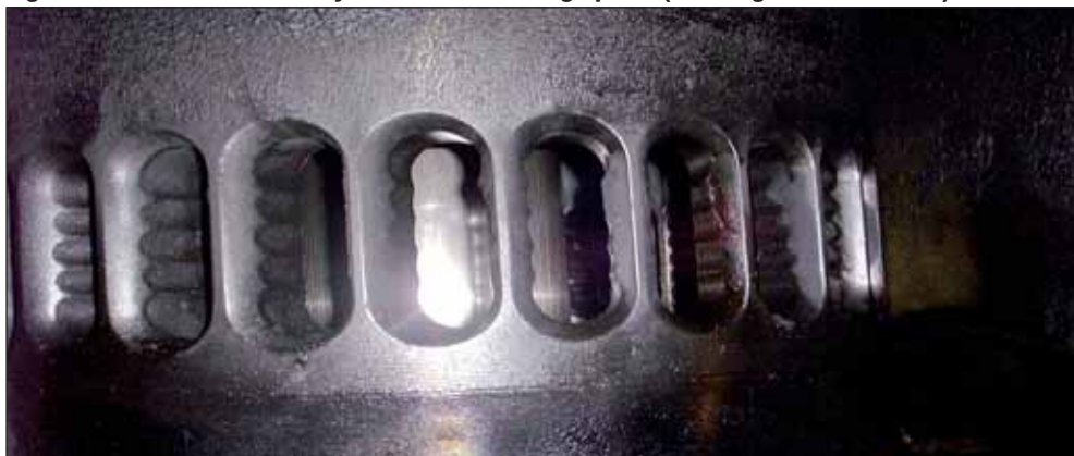
Figure 11: Number four cylinder liner scavenge ports (scavenge manifold side)
