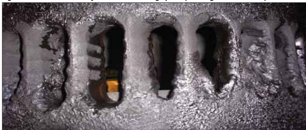
Figure 12: Number five cylinder liner scavenge ports (scavenge manifold side)
