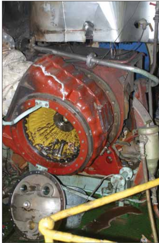
Figure 25: Opposite side of the second failed turbocharger, showing the exhaust inlet casing
