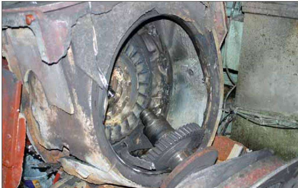
Figure 5: Failed turbocharger 12 February 2003
