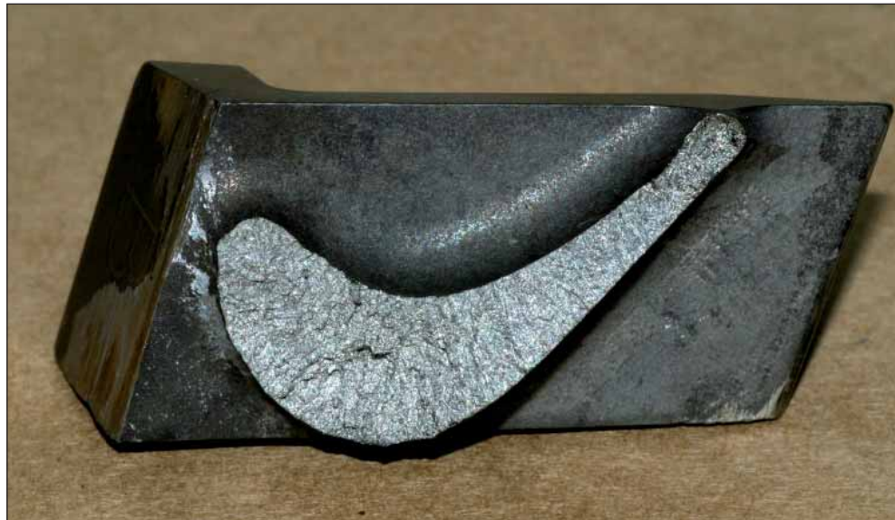
Figure 15: Same blade as fig. 14, cleaned and showing a uniform fracture typical of gross bending overloads
