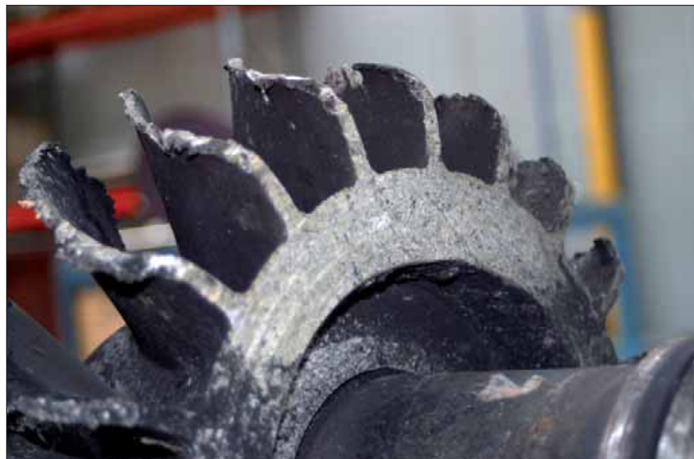
Figure 10: Rear face of the inducer element showing circumferential scoring consistent with continued rotation after the failure of the impeller disc
