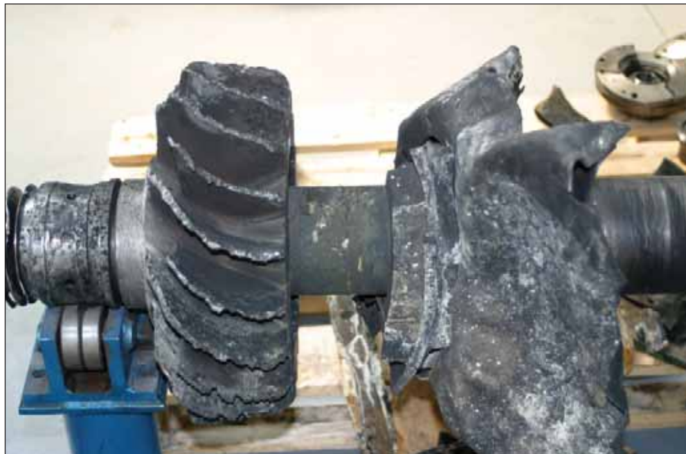
Figure 8: Compressor end of the turbocharger shaft. Missing the impeller disc
