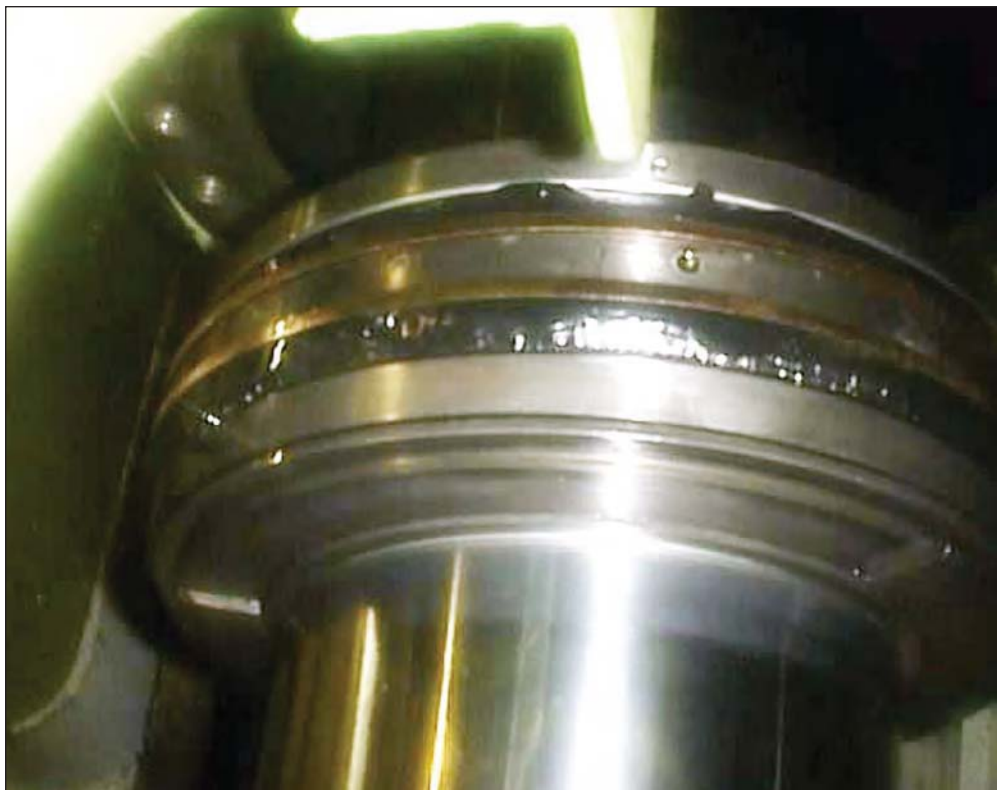
FIGURE 8: Starboard ram piston showing damaged seal rings
