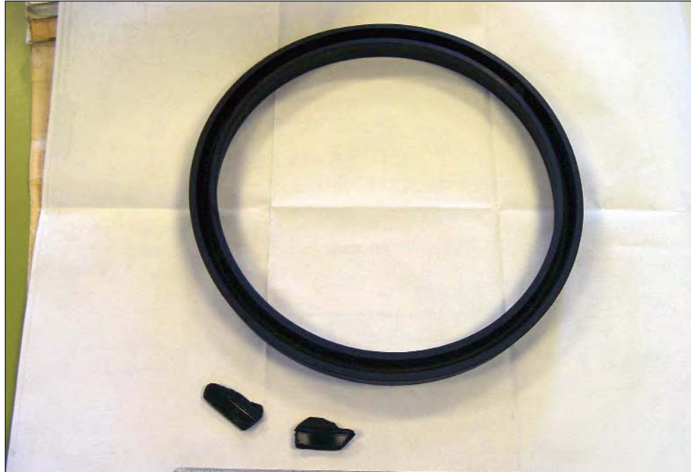
FIGURE 7: Piston seal and debris
