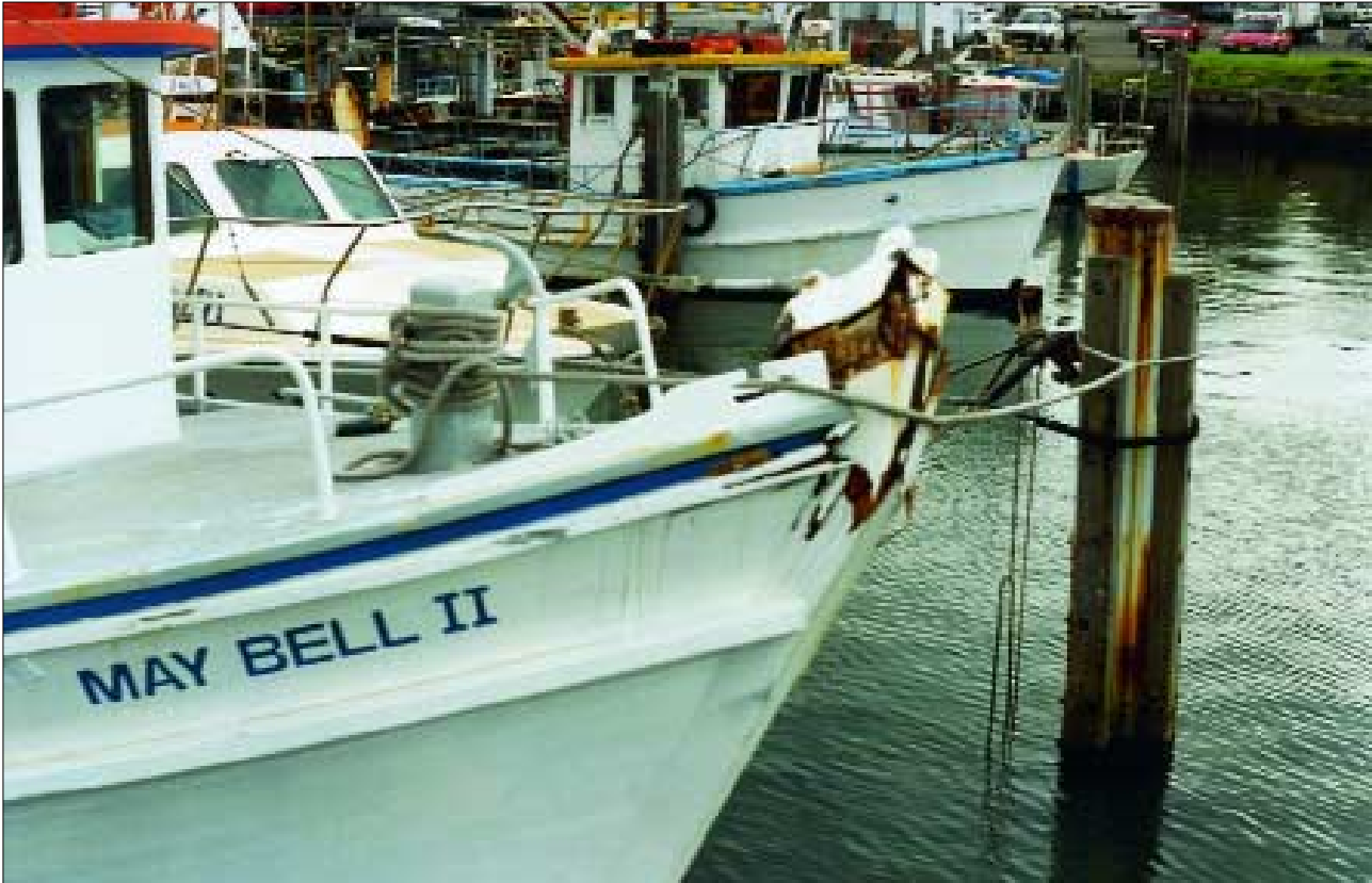
FIGURE 3 May Bell II , bow damage
