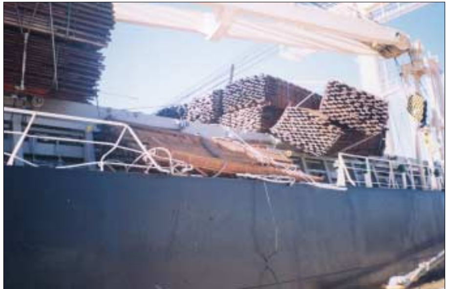
Figure 4: Deck cargo shown after shifting
