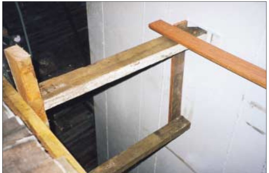
Figure 5: Lower hold cargo secured after incident
