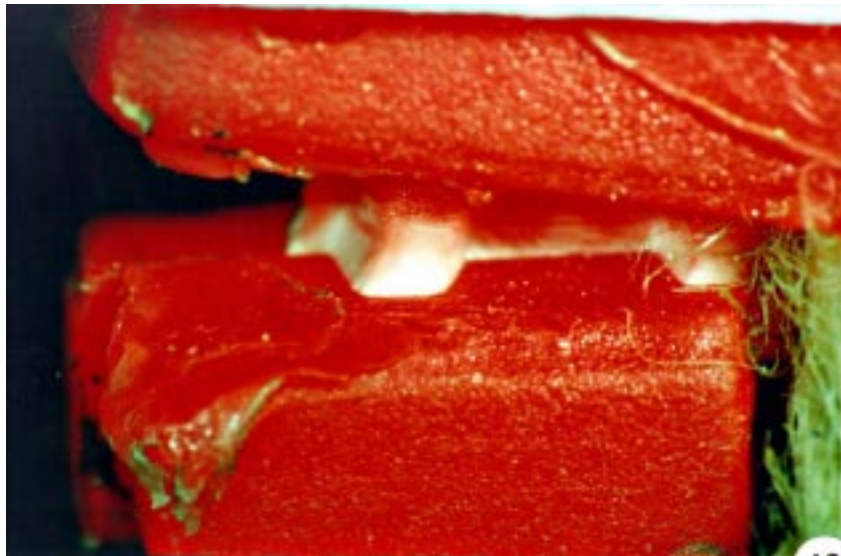
Figure 7 Macro examination of seal no. 0064801 showing tamper damage
