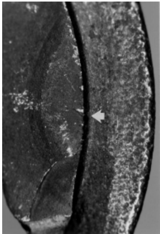
Figure 4. Detailed view of the site of primary fatigue crack initiation.
