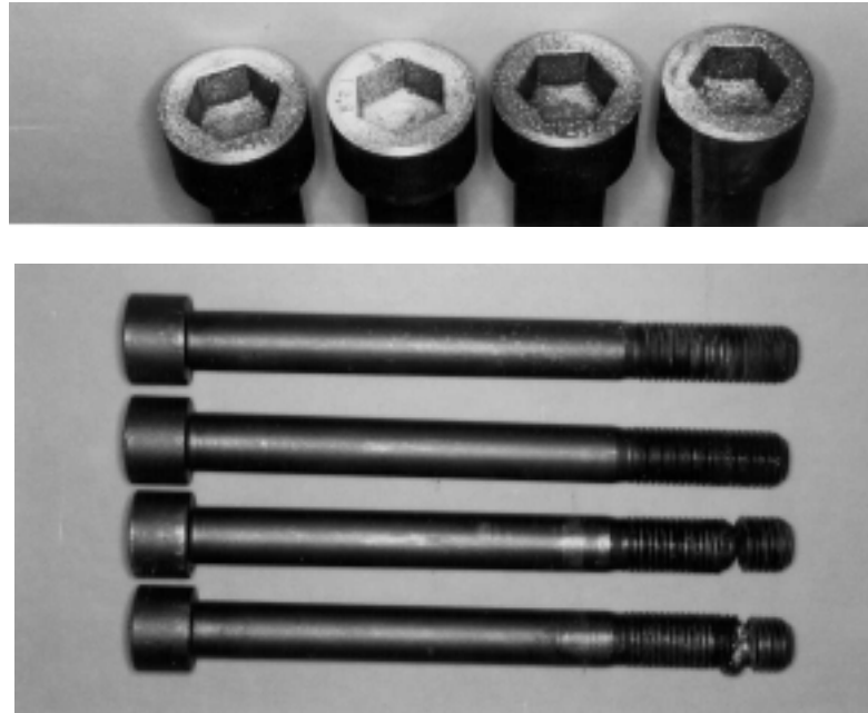
Figure 2. Cap screws from the failed pulsation damper filter/bypass hydraulic pump joint, as received.
