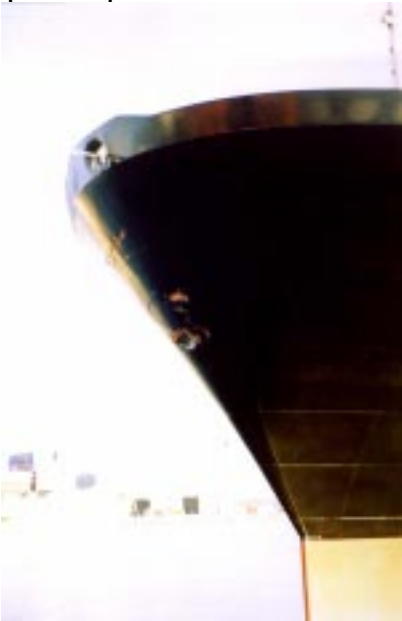
P & O Nedlloyd Sydney damage to bow
