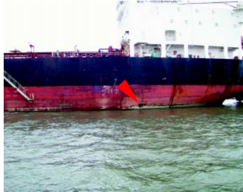
Location of holed shell plating on Barrington
