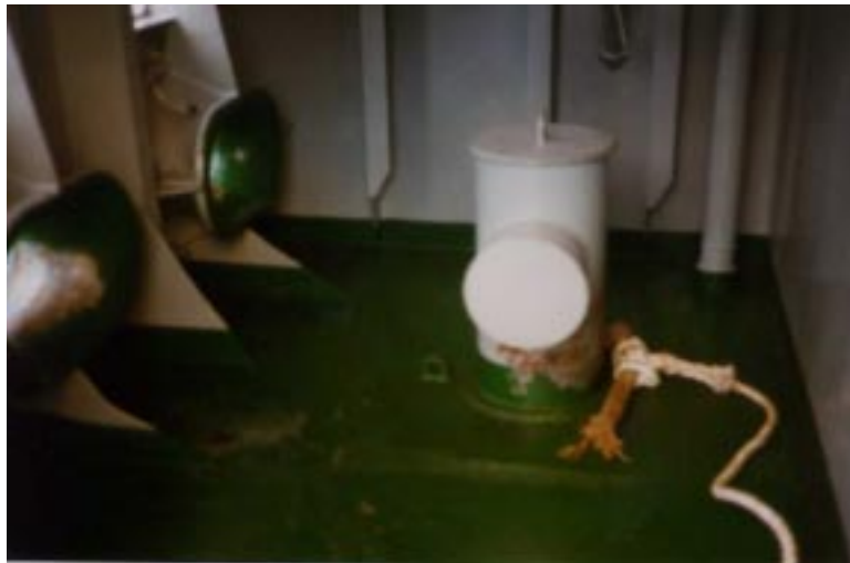
Photograph of bollard, piece of grommet and messenger
