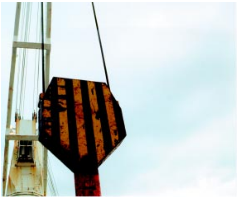
Cape Arnhem No.2 crane block showing rotor blade contact
