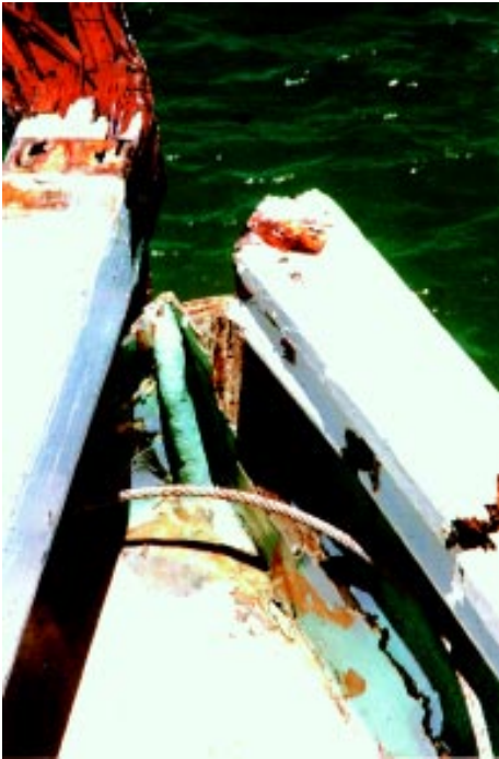
Damage to Moonshot's Bow
