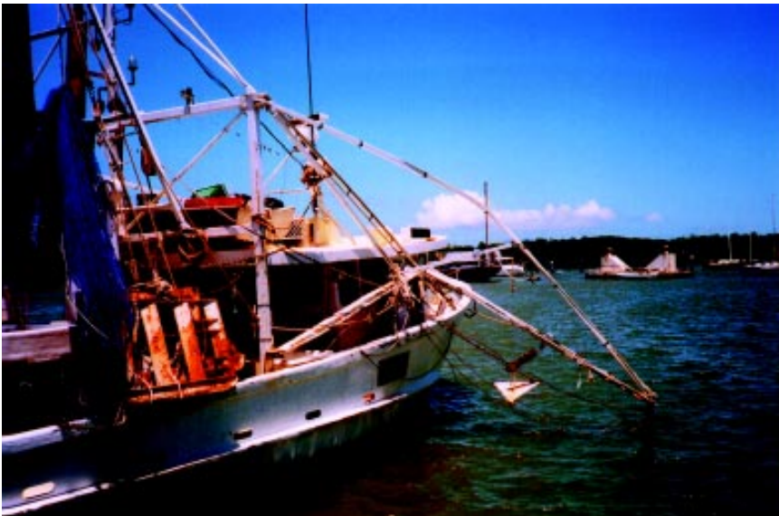
Damage to Moonshot's Starboard Outrigger
