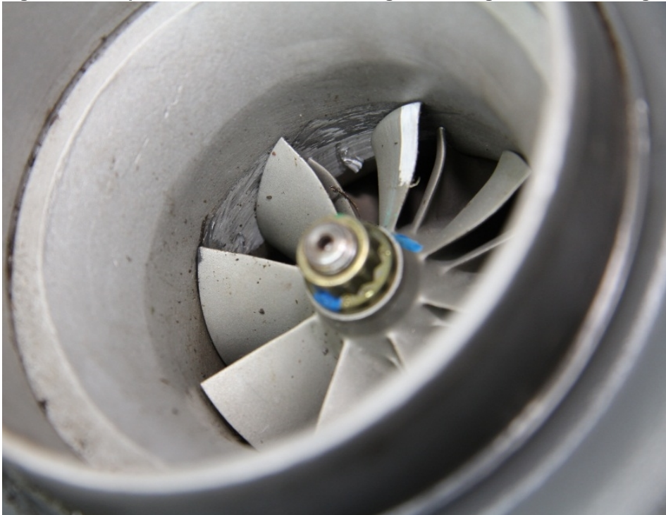
Figure 5: Compressor section of turbocharger showing rotational damage
