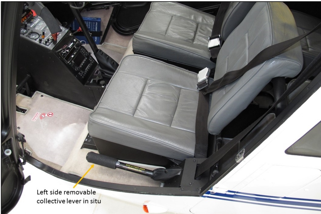
Figure 8: Typical R44 cockpit flight controls showing the removable left collective lever
