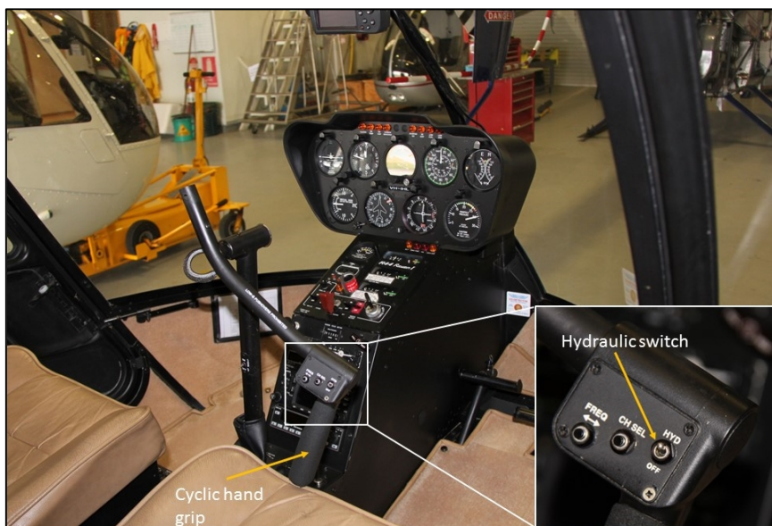
Figure 5: Typical R44 cockpit flight controls, pilot’s cyclic (left cyclic hand grip removed)
