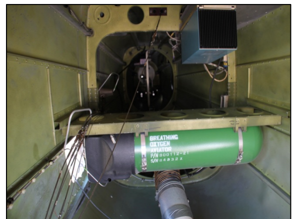
Figure 5: Rear fuselage area showing the oxygen bottle installation
