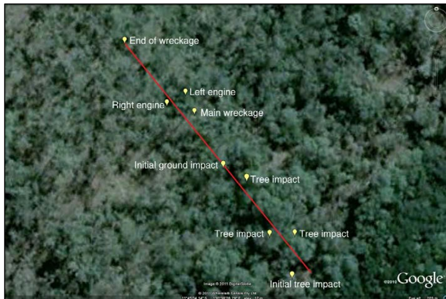
Figure 3: Overview of wreckage trail
