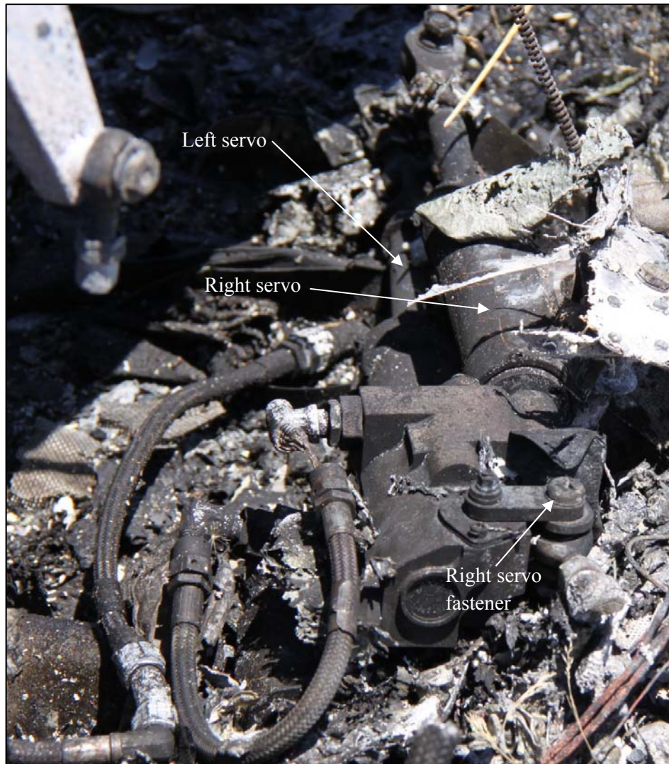
Figure 13: Right-front, left-front and exemplar hydraulic-boost servos
