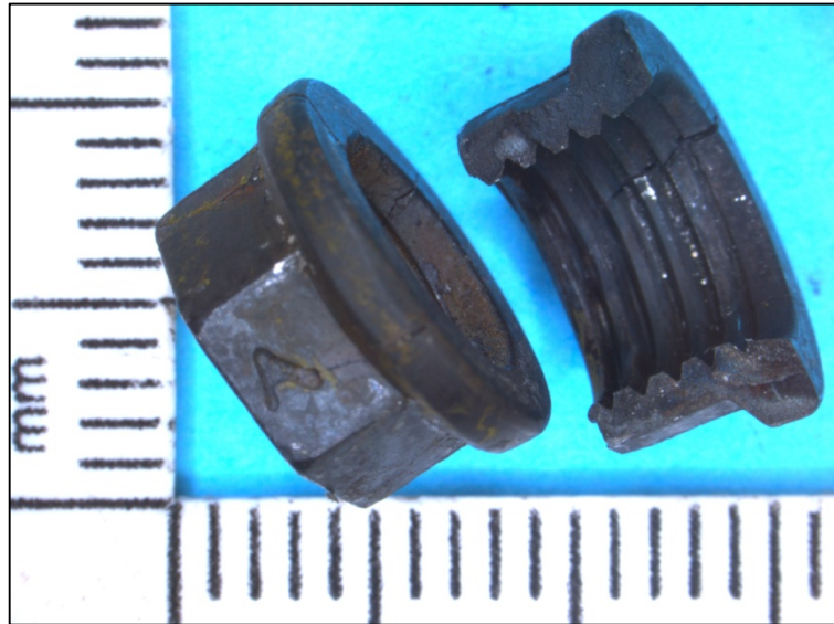
Figure 15: Cracked self-locking nuts
