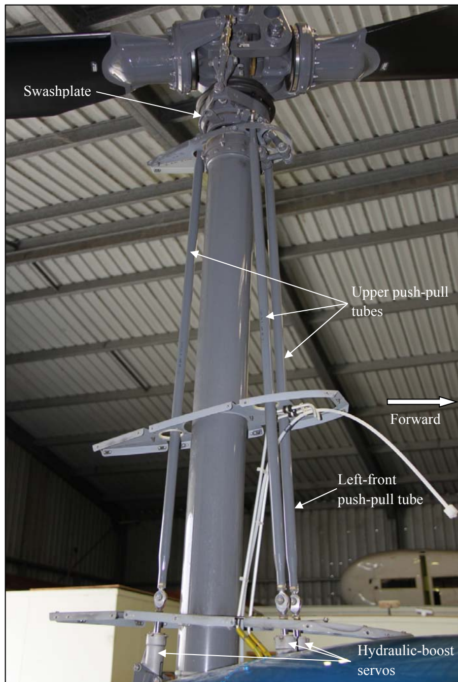
Figure 4: Main rotor flight controls (cowls removed for clarity)
