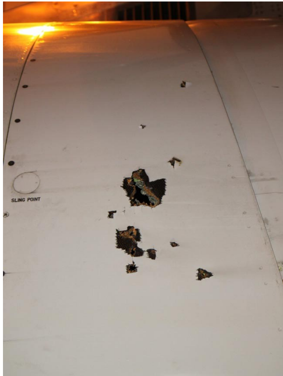
Figure 3: Punctures in nacelle, left side
