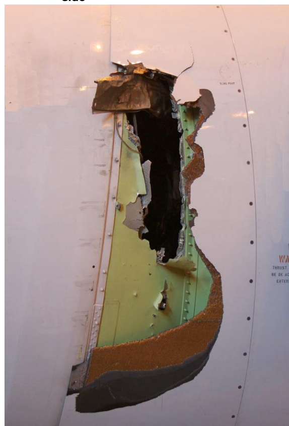
Figure 2: Perforation in the engine nacelle, right side
