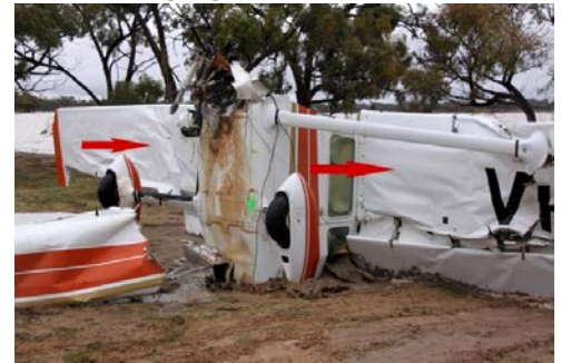
Figure 5: Lower wing surfaces with the hydraulic buckling damage highlighted
