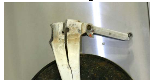
Figure 7: Nosewheel unit showing damage to the mounting collar
