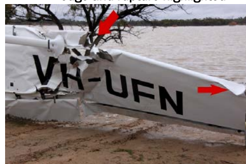
Figure 4: Left wing with flattened leading edge and rupture highlighted
