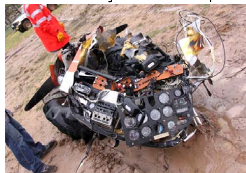
Figure 2: The engine, propeller and firewall assembly and instrument panel
