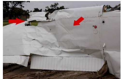
Figure 6: Upper surface of the left wing, showing the ruptured section and adjacent scoring and paint transference
