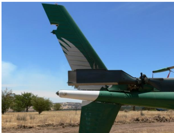
Figure 2: Damage in relation to tail rotor
