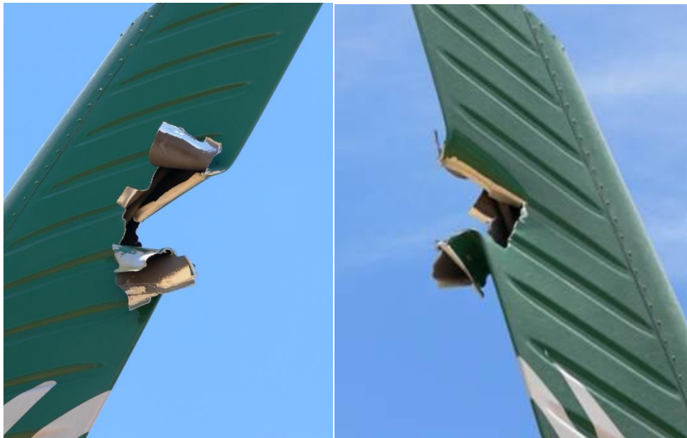
Figure 4: Damage to the vertical fin of NFO as viewed from the left and right sides
