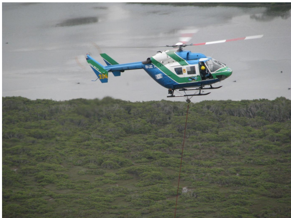
Figure 6: Showing LXC operating with a long line, with the pilot leaning outwards through the door opening, looking downwards, and ‘flying the bucket’
